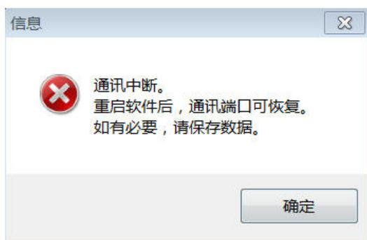
“正在通信时断开通信电缆”的错误弹窗
