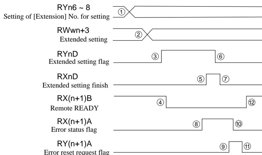
\* Note: Proceed to the next processing only after confirming that the "remote READY" RX(n+1)B is turned ON.
